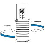
coming into the Dosmatic injector: i.e. adjustment at 1% = 1:100 = 1 volume of concentrate + 100 volumes of fluid entering the injector. **Check your manual for specific setting by model.**
